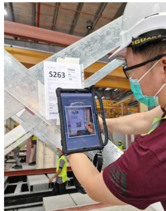
SPS-Flow allows users to quality control both products and processes by scanning the modules' unique QR codes.
